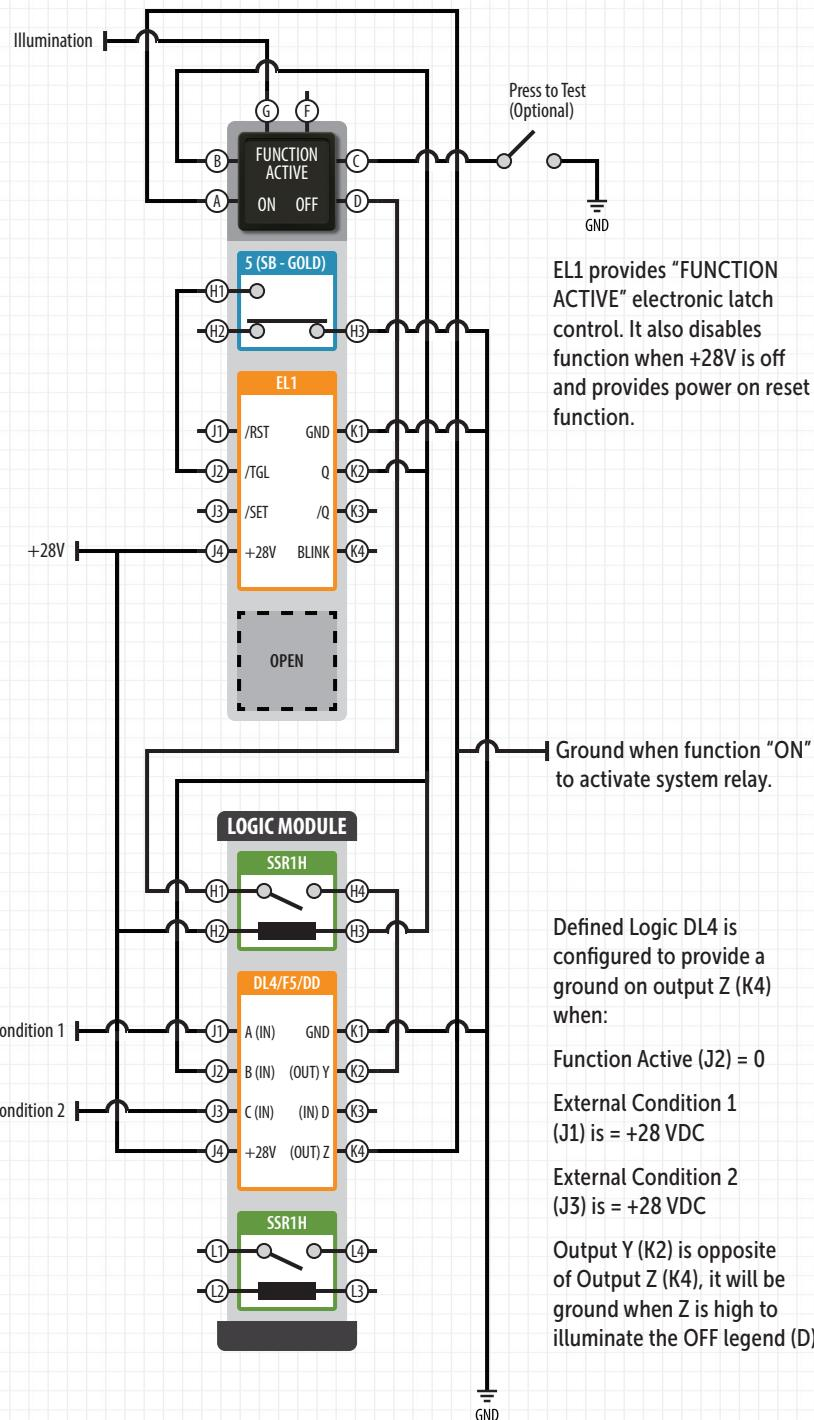
EL1 provides "FUNCTION ACTIVE" electronic latch control. It also disables function when +28V is off and provides power on reset function.
