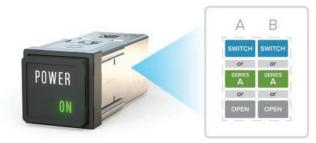
VIVISUN Compact bodies have two available positions (A and B in the diagram above). Compact bodies can contain up to two Series A components. An electromechanical switch pole can be used in place of a Series A component. Compact bodies cannot accommodate Series C, Series N or Series R NEXSYS components. Unoccupied positions will be configured with an Open spacer.
