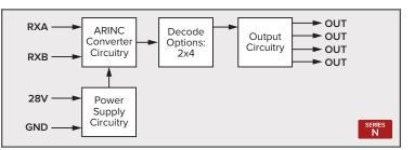
Series R (12 pin) SR429/4D: The decoding of two bits (2x4) producing four Decoded Outputs plus two Discrete Outputs based on decoded input and two unrelated Discrete or Failure Outputs for a total of eight outputs.
