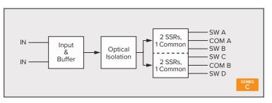
Three Switch Single Common, One Switch Single Common: Three (3) SPST contacts (or switches) connected to one common and one (1) SPST contacts (or switches) connected to another common.
