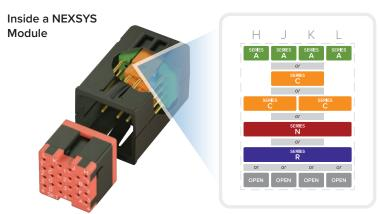
NEXSYS Modules have four available positions (H, J, K, and L in the diagram above). Modules can contain (a) up to four Series A components; (b) a single Series C component with up to two Series A Components; (c) two Series C components; or (d) a single Series N or Series R component. *See page 12.*
