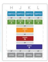
VIVISUN High Capacity bodies have four available positions (H, J, K, and L in the diagram above). High Capacity bodies can contain (a) up to four Series A components; (b) a single Series C or Series N component with up to two Series A components; or (c) a single Series R component with a single Series A component. An electromechanical switch pole can be used in place of a Series A
